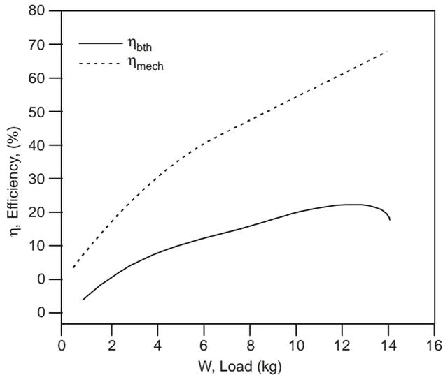
Fig. 2. Engine Performance for JCB-40 blend.
